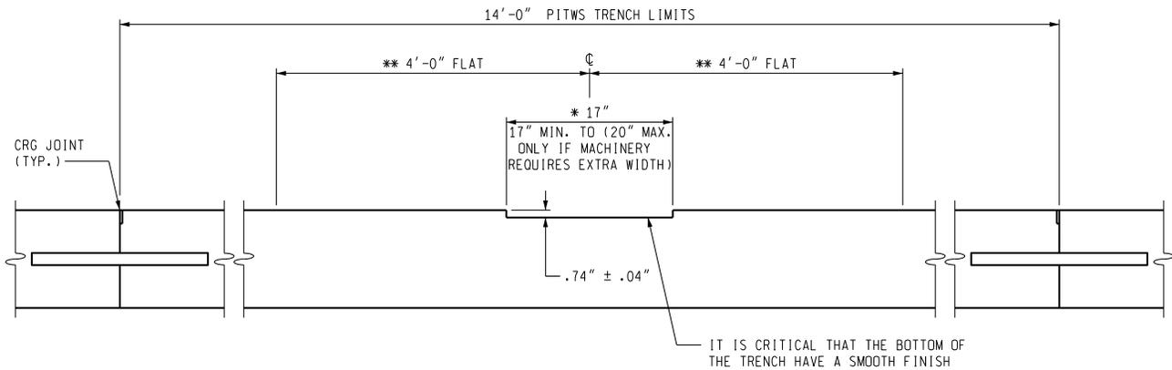
1. MACHINE CUT TO  $\frac{5}{8}$ " WITH 17" CUTTING HEAD
